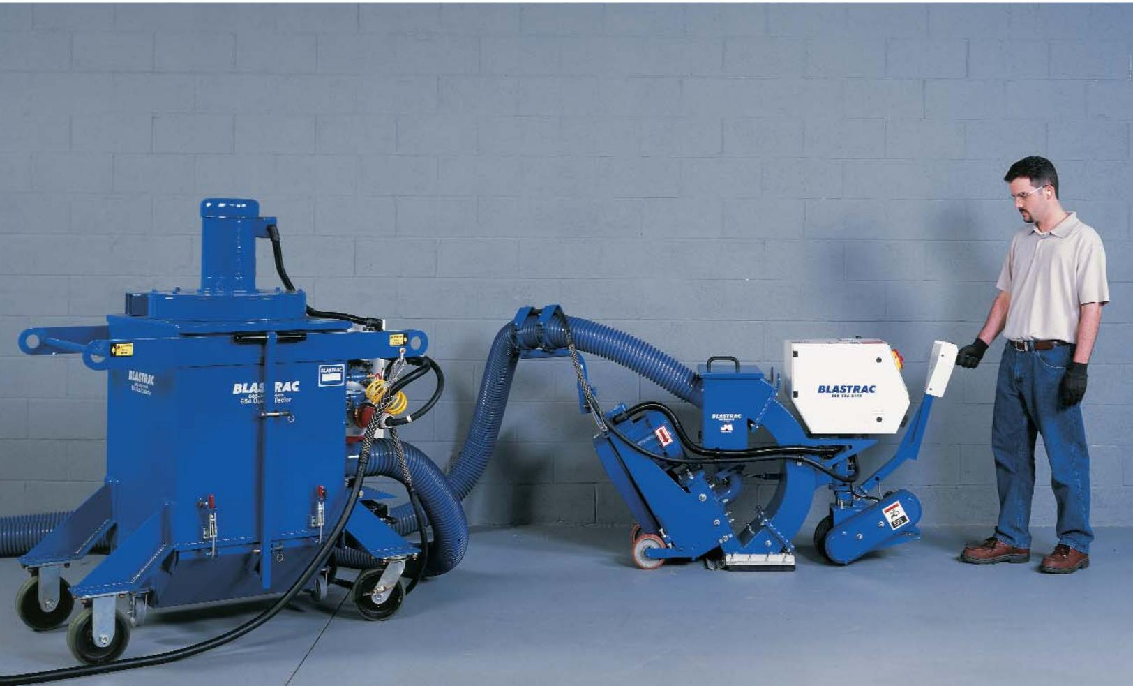
Blastrac® shot blasting is a cost-effective and environmentally friendly method for preparing concrete and steel surfaces. It is the surface preparation method recommended by most coating manufacturers.
